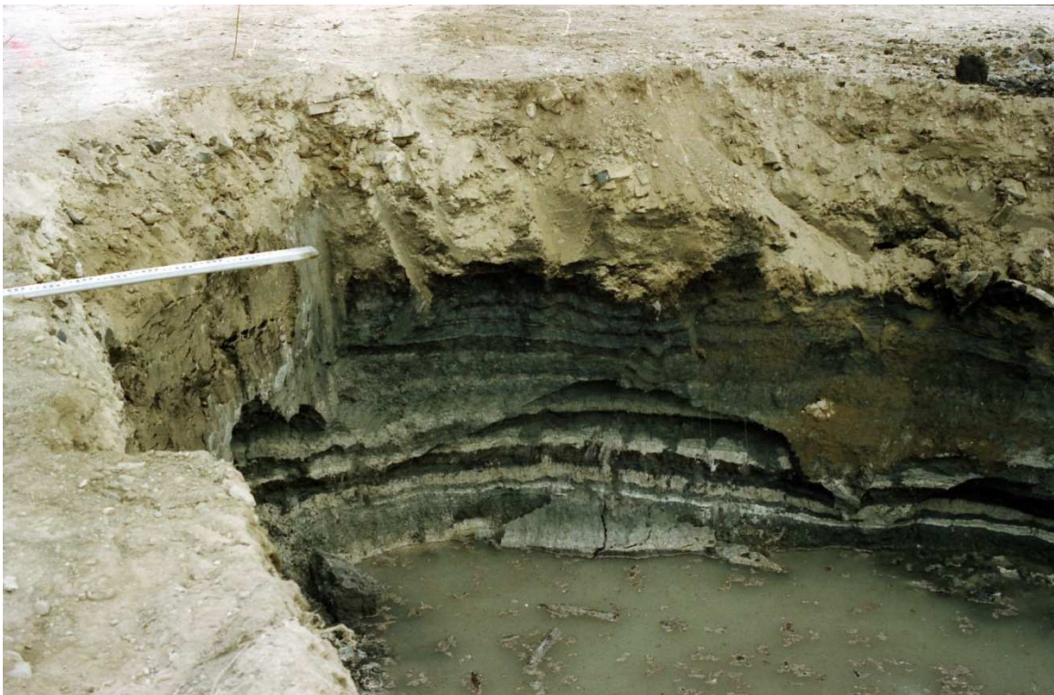
Figure 2 Interlayered very soft clay, peat, ash, and shells (~1m visible) beneath imported fill
